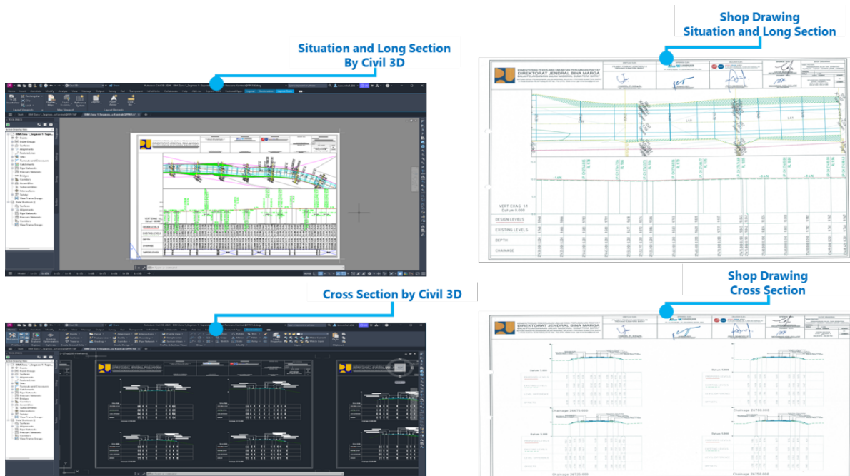
Figure 9. Output 3D shop drawing Highway from civil 3D
