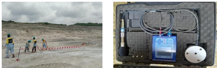
Figure 2. Survey and field measurement activities (a) and the Micromate Vibration Measurement Tool (Purwaningsih, A. 2023) (b)
