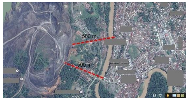
Figure 6. Safe Blasting Distance from Settlement (PT Semen Baturaja (Persero) Tbk., 2022)
