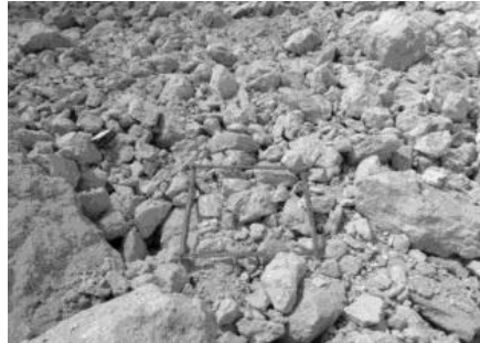
Figure 7. Limestone Fragmentation SampleBlasting Results in Block 49
