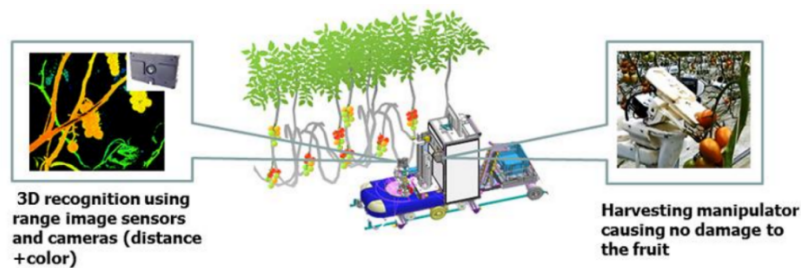
Figure 4. 3D sensors to action generated Machine Learning on Urban Plantation (lab Scale)
