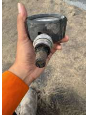
Figure 1. Pressure gauge there is dirt and dust that accumulates
